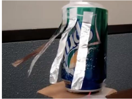
Figure 3: The effect of charge repulsion on aluminum foils in the Van de Graaff generator.
