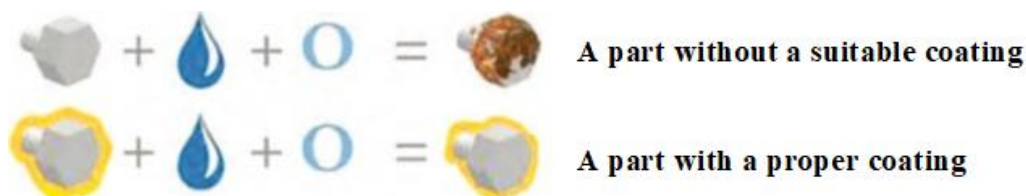
Figure 2 - Demonstrated efficacy of a protective coating in preventing corrosion on a metal screw (2004, EcoCortec Corporation)
